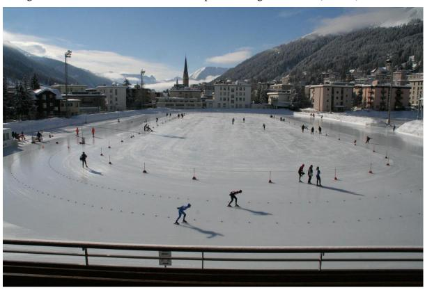
national Skating Union (ISU). The standard track, 400 meter to the lap, laid out on the Davos open air natural ice rink has the inner and outer curves with radii of 25.5 and 29.5 meters respectively with a warm up track.
